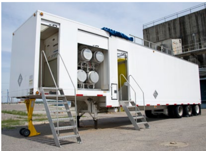
Five steel tanks (above), each capable of holding 16,000 gallons of liquid, are being prepared for shipment to Japan to potentially store contaminated fluid. The Radioactive Liquid Transport Assembly (below), used to sample and analyze contaminated liquids, will be provided as well.
