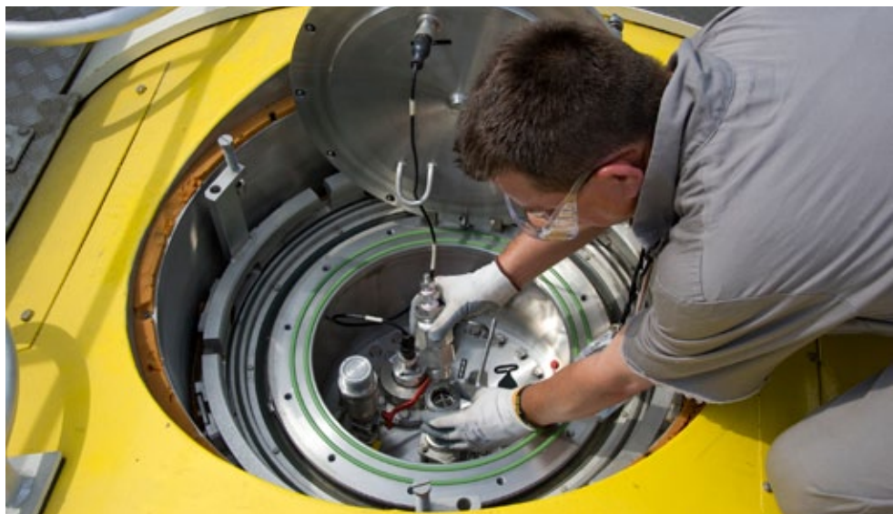
An SRNS operator tests components within a port used to access the interior of a 1,000 gallon tank housed within a mobile lab known as a Radioactive Liquid Transport Assembly soon to be transported to Japan.
