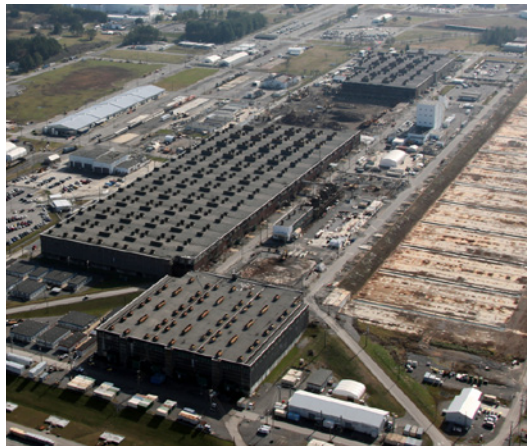
(Top) SRNS recently loaned the 94-ton 385C Caterpillar Excavator to URS CH2M Oak Ridge to assist with the K-25 demolition project at the East Tennessee Technology Park. (Above) Aerial view of the K-25 Building. The west wing has been demolished, while demolition and cleanup activities continue on the east wing.
