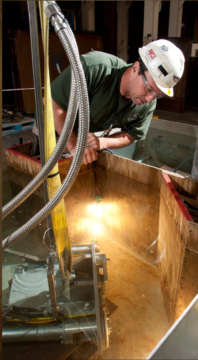
Photo (left and on cover): SRNS Construction Millwright Craig Usher observes preparations for a mock-up demonstration of the submersible pneumatic saw at a simulated basin.
