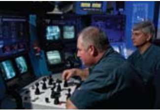
Operating the Hot Canyon Crane to insert uranium material into the 6.4D dissolver
