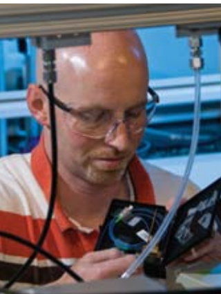
Performing research and development on novel trace gas optical sensors to determine impurities in hydrogen process streams
