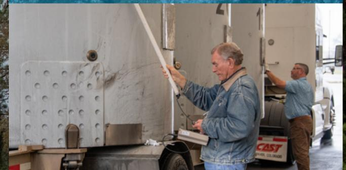
Shipping containers are surveyed to ensure no radiation is present before leaving SRS.
