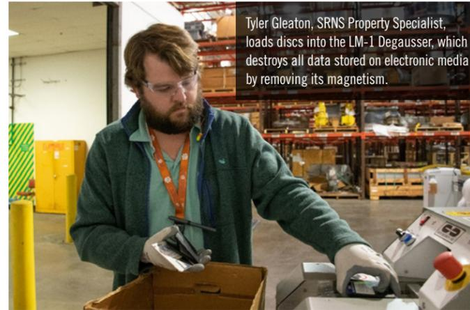
Tyler Gleaton, SRNS Property Specialist, loads discs into the LM-1 Degausser, which destroys all data stored on electronic media by removing its magnetism.
