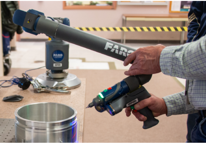
The FaroArm has the capability to scan 600,000 dimensional points per second.
