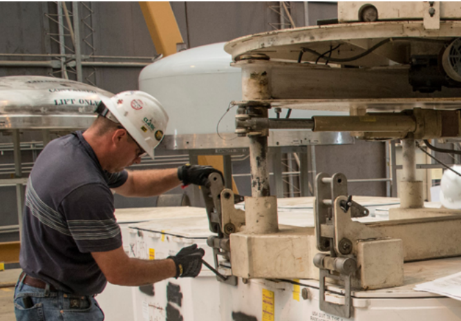
An SRNS employee safely packages transuranic waste in specialized containers for shipment to the Waste Isolation Pilot Plant.
