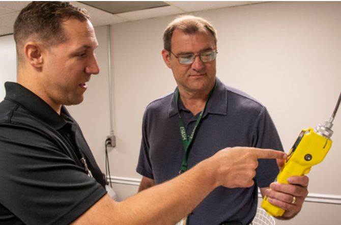
SRNS Senior Industrial Hygienist Chris Wells instructs Chris Frazier of the SRS Ft. Gordon Job Shadowing Program on the use of a volatile organic compound meter to monitor the air in a building that is undergoing a roof replacement.
