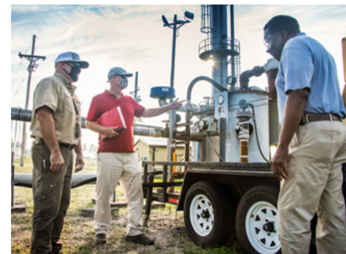
Mechanic Todd Cockrell (left), Engineer John Bradley (center) and Project Manager Joao Cardoso-Neto plan the removal and dismantlement of a now-unneeded high-vacuum soil vapor extraction unit, also pictured below.
