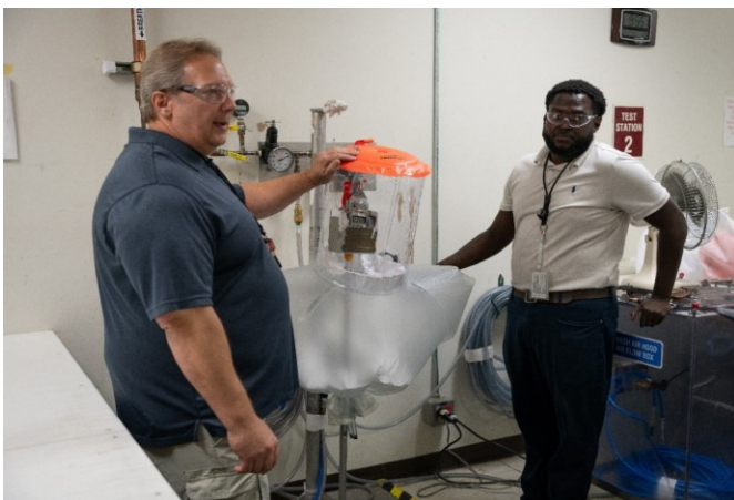
Respirator Equipment Facility personnel Jeffrey Detiege (left) and Aaron Beverly demonstrate how the plastic suits are tested for air flow, leaks and other deficiencies.
