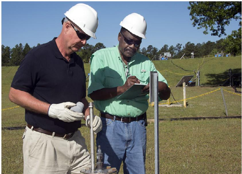
*John Bradley, Design Authority Engineer (left) and Joao Cardoso-Neto, Upper Three Runs Project Manager, both with the SRNS Area Cleanup Projects organization, inspect a BaroBall™ unit. This remediation technology operates completely on natural changes in barometric pressure to pump chemical contaminants from the subsurface.*
