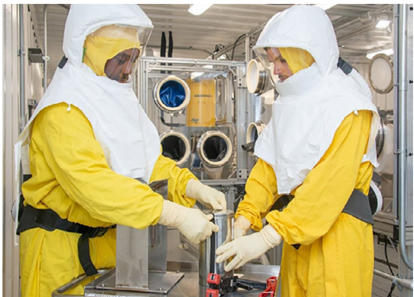
Savannah River Site radiation protection employees don protective equipment while working in a glovebox. Gloveboxes are structures with ports containing gloves that allow waste handlers to safely work with radioactive material.
