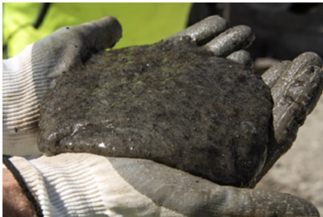
Workers mixed more than a million pounds of iron filings with a food-grade, starch-like material, shown here.
