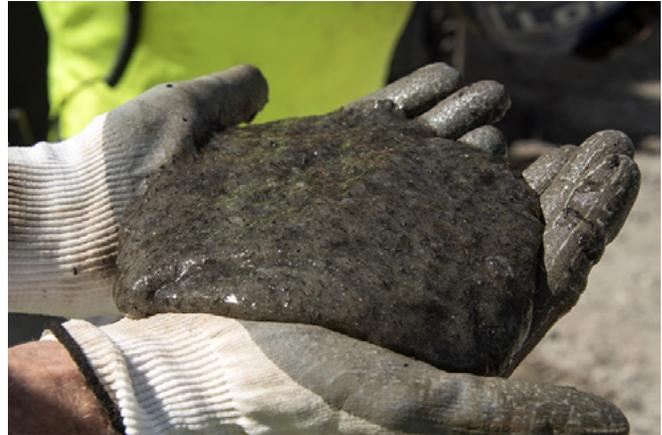
*Workers mixed more than a million pounds of iron filings with a food-grade, starch-like material, shown here. The material was injected into 22 wells at the Savannah River Site to create a long and continuous iron wall that acts as a giant metal filter of contaminated groundwater.*
