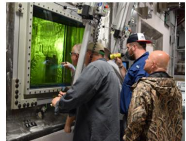
*Operators use manipulators and basic hand tools to conduct initial disassembly of the cutter head inside the TRP module. Lead-plated glass provides radiation shielding. Photography was taken prior to the latest COVID-19 guidelines reinstating mask requirements for vaccinated employees.*
