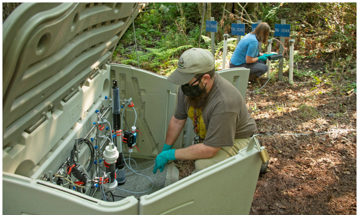
Savannah River Ecology Laboratory soil scientists Jeffrey Lott, left, and Christina Logan monitor experimental test equipment used to remove iodine-129 from groundwater at the Savannah River Site. The equipment is part of a one-of-a-kind system developed at the site for this study.
